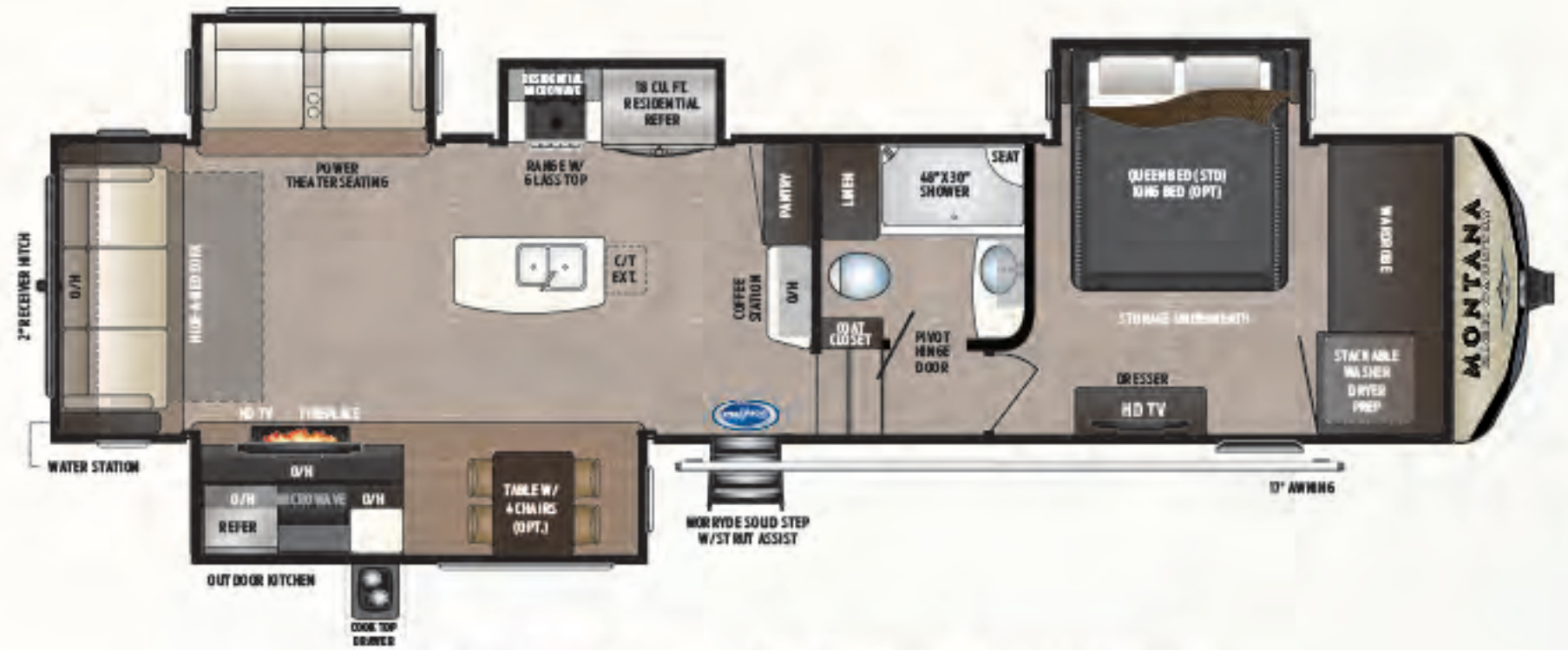
344/345RL Rear living room w/ outside kitchen RV REFRIGERATOR RES. REFRIGERATOR Weight: 11501 LBS. | Length: 36' 4"
