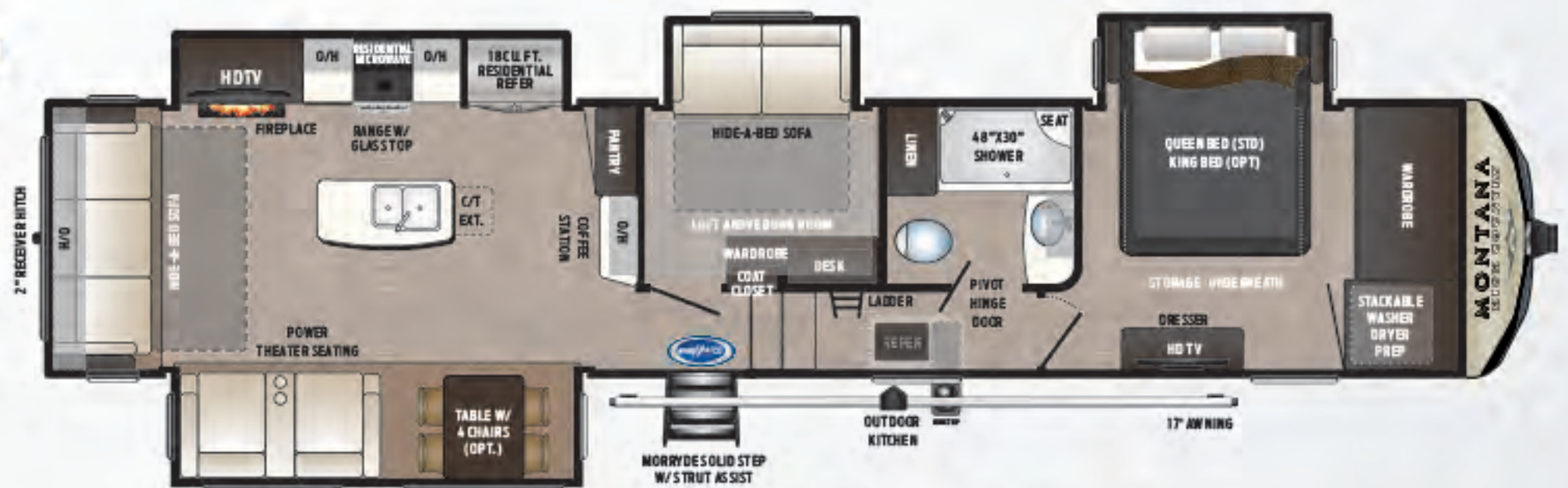
384/385BR Bonus room w/loft and outside kitchen RV REFRIGERATOR RES. REFRIGERATOR Weight: 12860 LBS. | Length: 40' 8"
